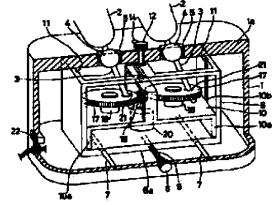
disks rotated horizontally. Both disks are provided on an elevating support plate, and the support plate is installed in a slide box capable of moving forward and backward in the case.
